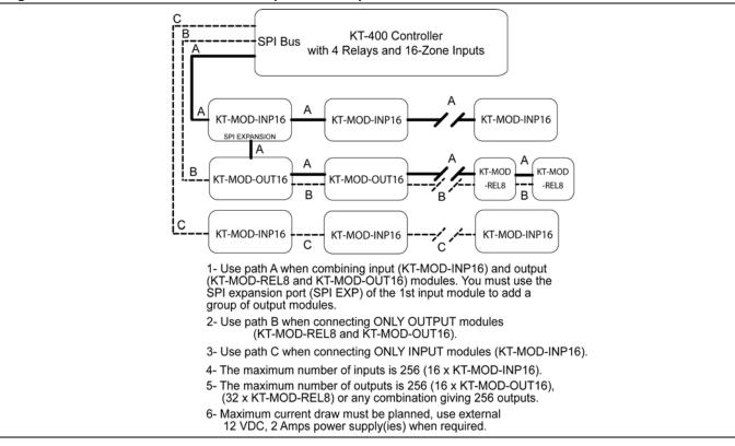
The number of expansion modules that can be connected to the KT-400 SPI expansion port, without an additional external power supply, can vary depending how much current is drawn from all the modules in the SPI chain.
